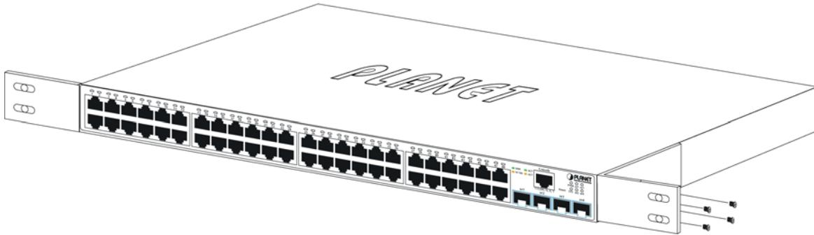
Figure 2-2-2: Attach Brackets to the Managed Switch.
