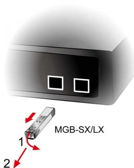
Figure 2-2-5: How to Pull Out the SFP/SFP+ Transceiver
