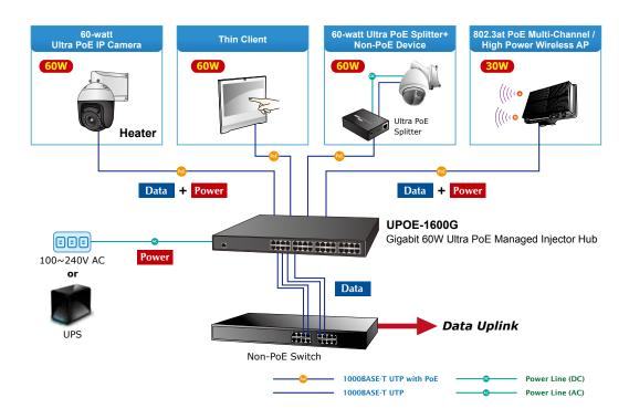
With data and Power over Ethernet from one unit, the UPOE-1600G can reduce power cable deployment and eliminate the need for dedicated electrical outlets on the wall, ceiling or any unreachable place.
