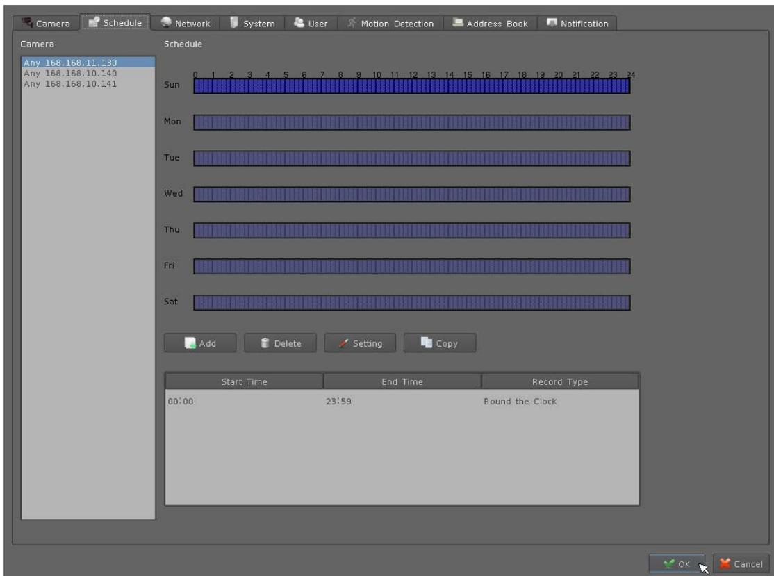
The interface shows a 'Schedule' tab with a list of cameras on the left and a 24-hour grid for each day of the week (Sun-Sat) on the right. Below the grid are buttons for 'Add', 'Delete', 'Setting', and 'Copy'. At the bottom, there is a table for recording settings.
