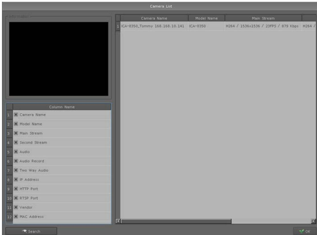
The screenshot shows the 'Camera List' interface. On the left, there is a 'Column Name' menu with 12 items, each with a checked checkbox:
