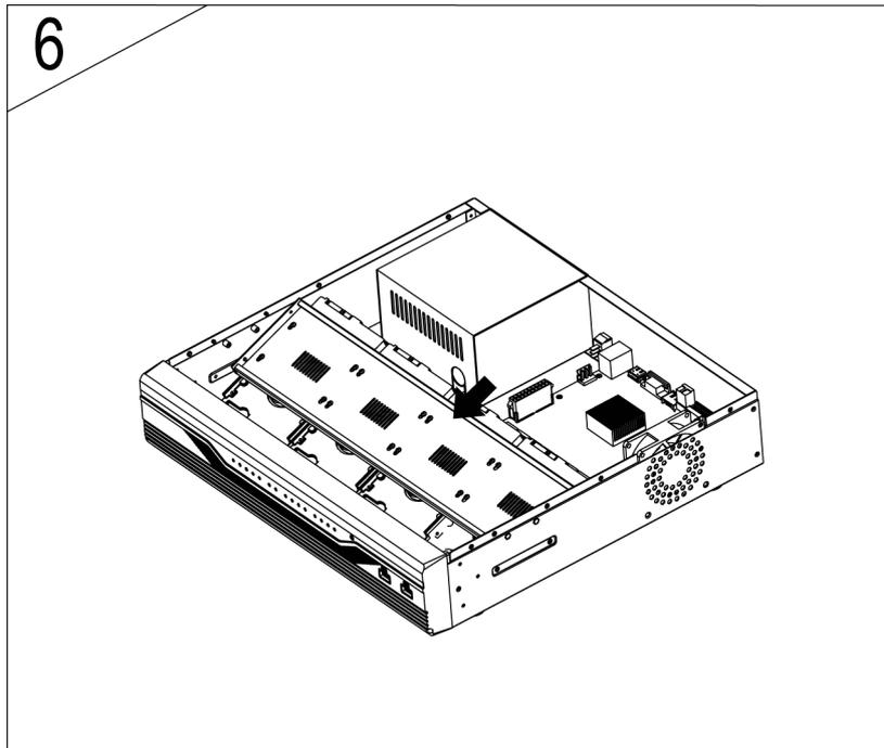
**7. Latch the fixed plates of hard drives and case with screw.**
