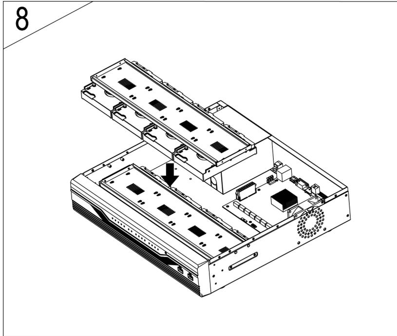
**9. Latch the fixed plates of hard drives and case with screws.**
