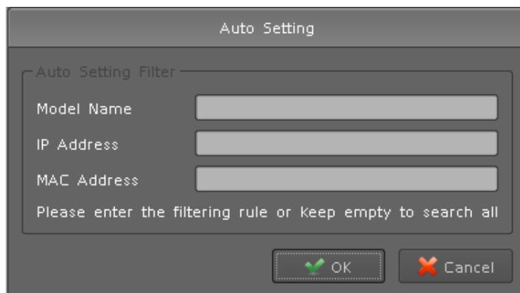
Auto setting could insert Intranet’s cameras even these cameras are located behind several switch hubs. Besides, you could directly insert cameras on NVR’s switch hub and then click the “Auto Setting”button to add them to system. Through “Auto Setting”function , you do not need to key-in any network IP address or sub-mask parameter. All you need to do is click the “Auto Setting”button to finish the job of inserting IP camera.
