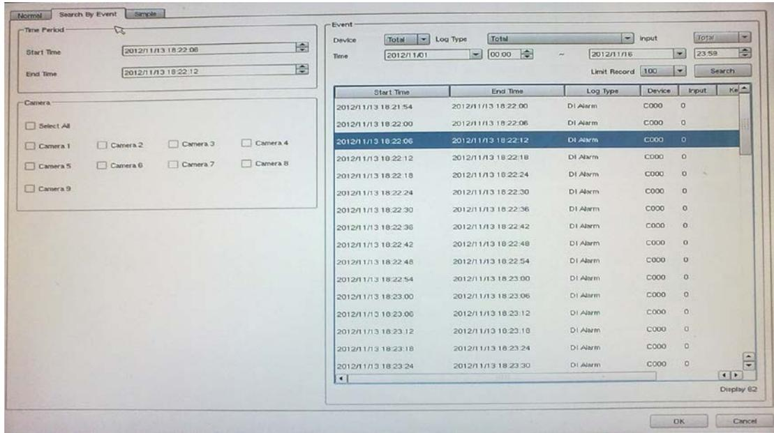
Input search filter first by clicking the “Search” button; the search result will display on the list as shown above. Select a log that you need to play back. System will fill the event period automatically, and select which cameras you need to play back together. Click the “OK” button when the search is done.
