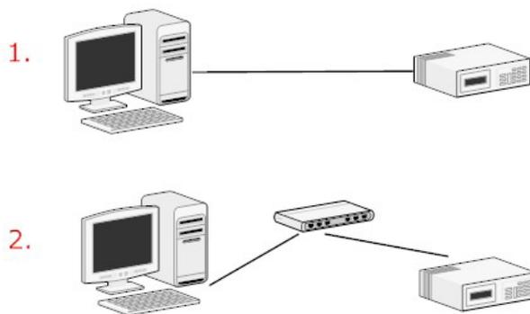
The PC that is connected directly to the NVR (or within the same local area network) should receive an IP from it. Simply access the NVR from your Web browser with NVR default IP address.
