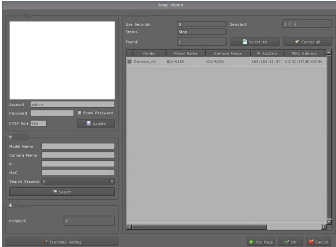
7. After setup wizard is finished, the NVR will ask the first login. The default login user name and password are both "admin".
