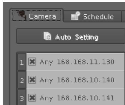
Check the box to make the camera available for video streaming; otherwise, the camera will be disabled if the check box is empty.
