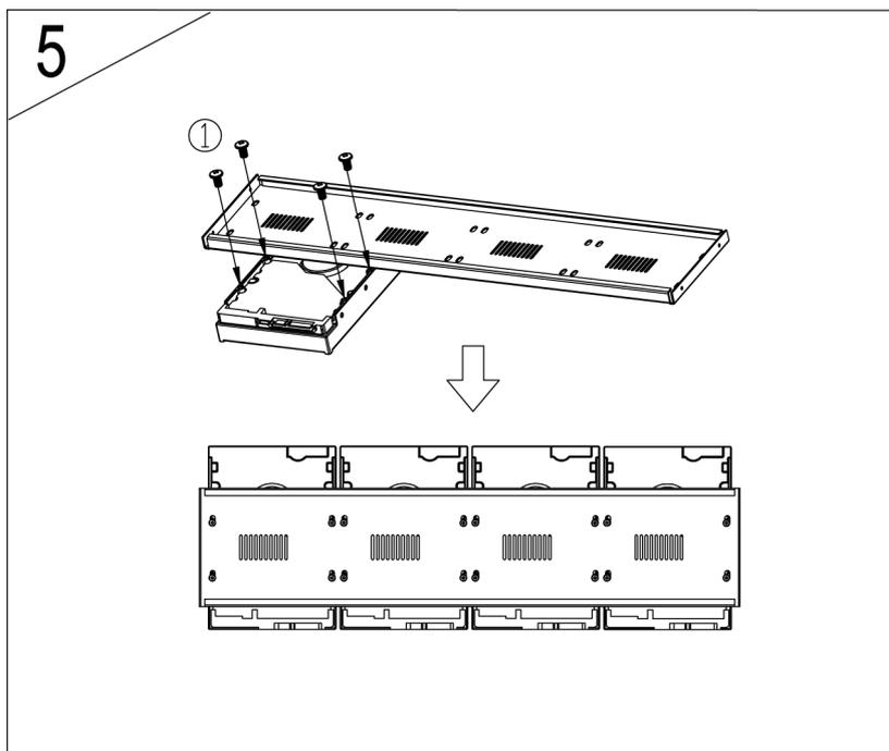
**6. Place back the bottom of fixed plates of hard drives.**
