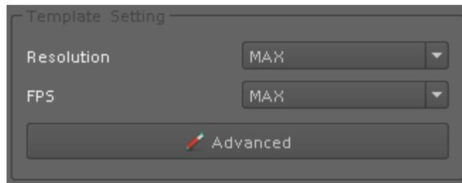
After the template has been confirmed, you will no longer need to set up parameter of camera again in most cases. You could set up the quick template from camera setting page and only need to set the camera’s resolution and frames per second. If you need to set up more details in template, please click the “Advanced” button to approach the template setting dialog.
