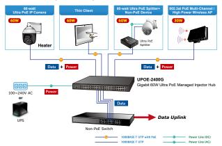
With data and Power over Ethernet from one unit, the UPOE-2400G can reduce power cable deployment and eliminate the need for dedicated electrical outlets on the wall, ceiling or any unreachable place.
