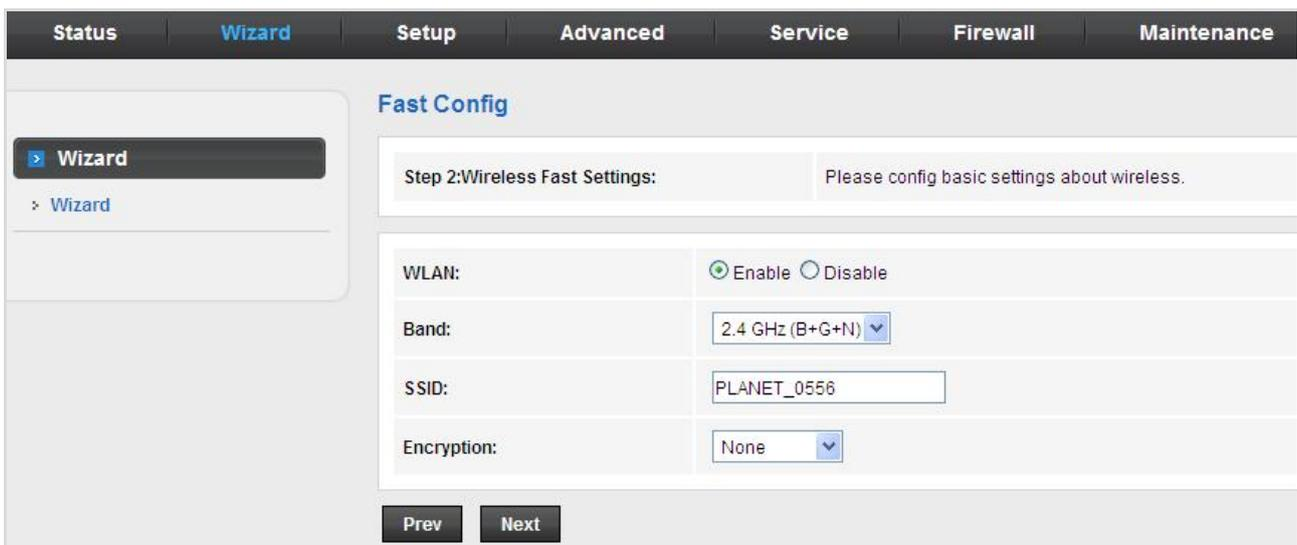
The screenshot shows the 'Fast Config' wizard interface at Step 2. The top navigation bar and sidebar are the same as in Figure 5-6. The main content area is titled 'Fast Config' and contains the following text: 'Step 2: Wireless Fast Settings: Please config basic settings about wireless.'. The configuration fields are: 'WLAN' (Enable selected, Disable), 'Band' (2.4 GHz (B+G+N)), 'SSID' (PLANET\_0556), and 'Encryption' (None). 'Prev' and 'Next' buttons are at the bottom.
