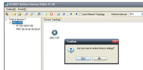
2.5: Press **"OK"** to complete the factory default procedure.
