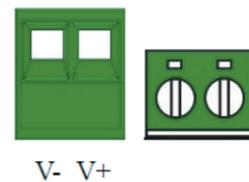
**Note** Please follow the DC power input symbol from the front panel of the IMG-110T -- insert positive DC power wire into **V+**, and negative DC power wire into **V-**. Otherwise, it will damage the device.
