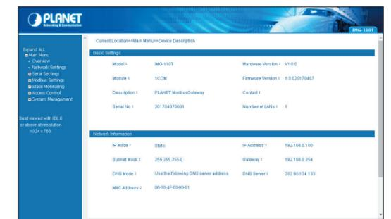
Figure 4-3: Web Main Screen of Industrial Modbus Gateway
