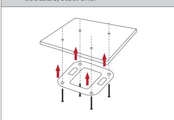
**Step 2:** Load the device into the mounting bracket, and be sure the device is mated with fixed screws. Then, lock the device in position and plug the Ethernet cable into the WNAP-C3220E.
