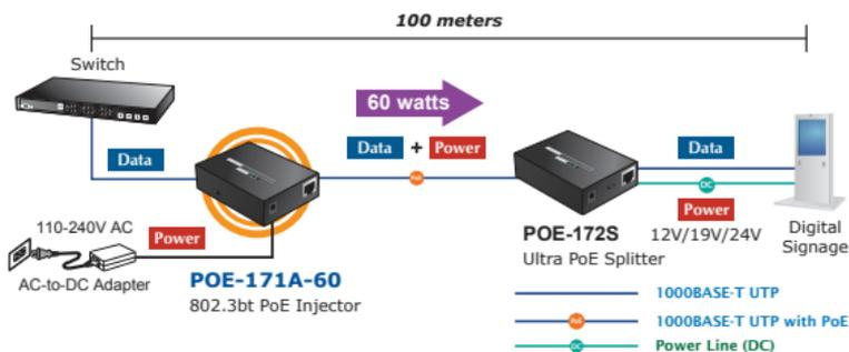
**Figure 4:** Connected Architecture over POE-171A series and POE-172S
