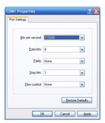
Figure 3-2: COM Port Configuration
