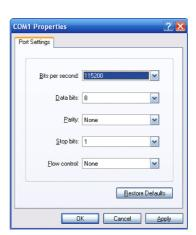
Figure 3-2: Hyper Terminal COM Port Configuration
