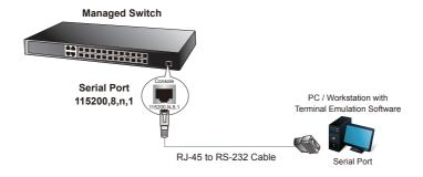
Figure 3-1: GS-5220-16S8C/GS-5220-16S8CR Console Connectivity
