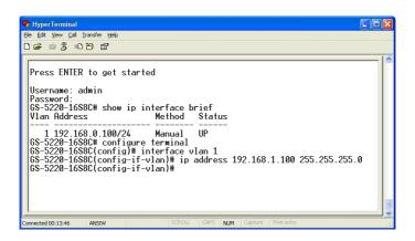
Figure 5-2: Configuring IP Address Screen
