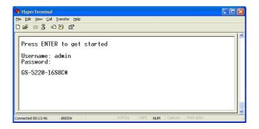
Figure 4-1: Managed Switch Console Login Screen
