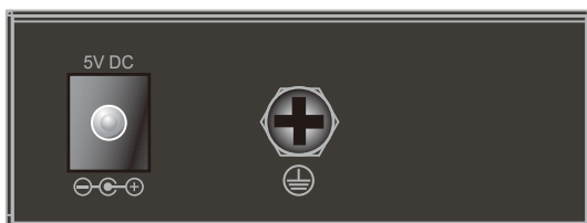
Figure 2-3: One DC jack for DC power input
