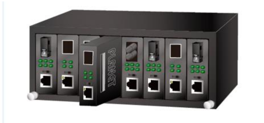
Figure 2-2: Insert Managed Media Converter into an available slot
