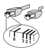
The standard RJ-45 receptacle/connector
