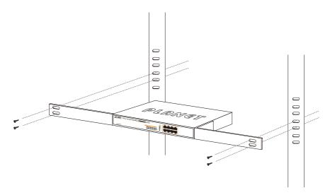
Figure 2-6: Mounting the Switch in a Rack
