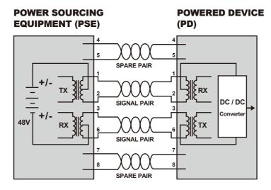
Figure 2 - Power Supplied over the Data Pins
