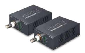
PLANET VC-205-KIT PoE over Coaxial Extender Kit is designed to extend IP Ethernet transmission and inject power over an existing coaxial cable for distance up to 1000m (3280ft) into PoE IP camera, PoE wireless AP and any 802.3af/at complied powered device (PD).
