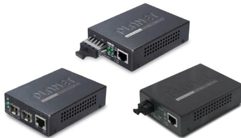
For the flexibility of all kinds of 10/100/1000Mbps Ethernet Media on RJ45 port and highly-stable Gigabit fiber performance, PLANET GT-802, GT-802S, GT-805A and GT-806A/B series and GT-1205A Gigabit Ethernet Media Converter extend communication distance with Gigabit performance via fiber optic cable. The GT-80x series and GT-1205A provide media conversion between 10/100/1000BASE-T and 1000BASE-SX/LX interfaces for various fiber optic applications.
