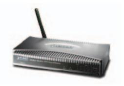
The PLANET VRT-401G is a 802.11g compliant Wireless VPN Firewall Router that is designed for sharing Internet connection to user's LAN and WLAN at the same time. It supports 64/128-Bit WEP (Wired Equivalent Privacy), WPA-PSK, WPA, WPA2 Encryption and MAC/IP filter access control for securing wireless network connection. The VRT-401G supports not only AP mode, but also AP Client, Bridge and WDS modes; in other words, it provides more flexibility for users to establish their wireless network.
