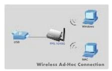
Work with the Wireless interface and configure the print server to "Ad-Hoc" mode. All wireless users can share the printer.
