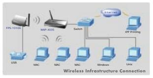
Work with Wireless interface and configure the Print Server to "Infrastructure" mode. All wired, wireless and Internet users can share the printer.
