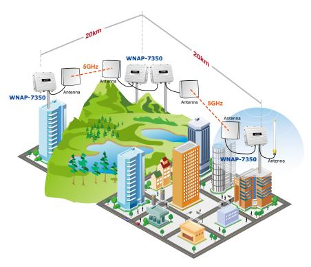
With built-in two N-Type Antenna connectors, the WNAP-7350 brings higher coverage and longer distance of wireless connection. The WNAP-7350 provides high output power with multiple adjust Tx controller, which allows CPE users to easily install and adjust the suitable value in appropriate locations. The WISP mode supported in the WNAP-7350 also enables CPE users to connect to Internet via local WISP provider conveniently.
