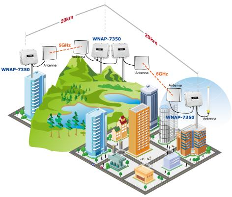
With two built-in N-Type Antenna connectors, the WNAP-7350 brings higher coverage and longer distance of wireless connection. The WNAP-7350 provides high output power with multiple adjust Tx controller, which allows CPE users to easily install and adjust the suitable value in appropriate locations. The WISP mode supported in the WNAP-7350 also enables CPE users to connect to Internet via local WISP provider conveniently.
