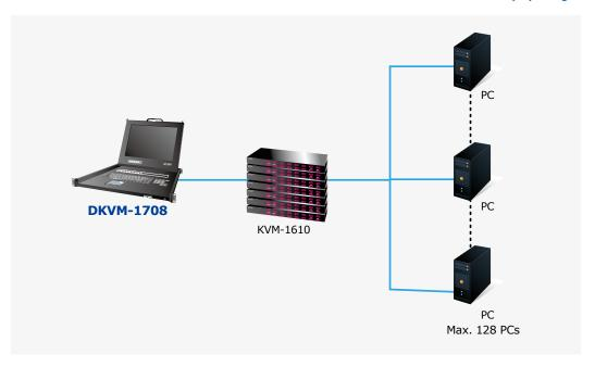
The Combo-Free KVM can be connected to any PC or server directly without concern of keyboard / mouse interface compatibility.
