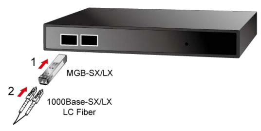
Figure 2-5 Plug in the SFP transceiver
