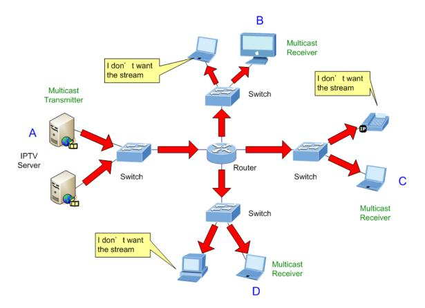
Figure 4-7-4 Multicast flooding
