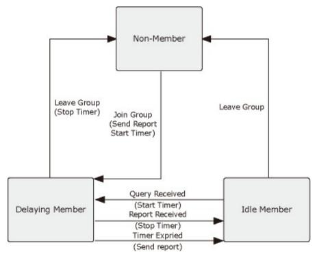
Figure 4-7-6 IGMP State Transitions
