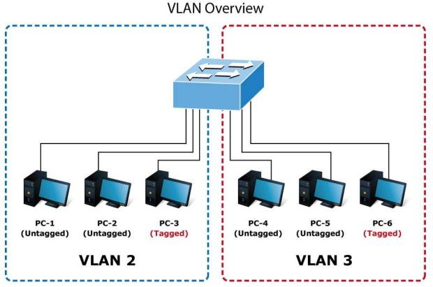
Figure 4-5-20 two separate VLAN diagrams
