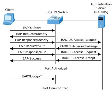
Figure 4-9-2 EAP message exchange
