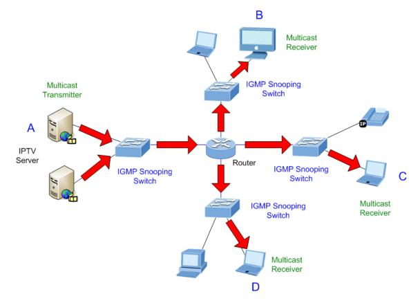
Figure 4-7-5 IGMP Snooping multicast stream control
