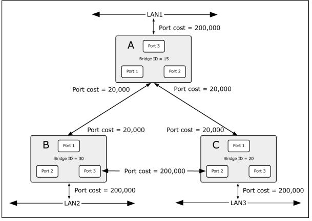
Figure 4-6-2 Before Applying the STA Rules
