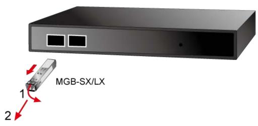
Figure 2-8 How to Pull Out the SFP Transceiver
