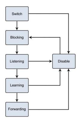
Figure 4-6-1 STP Port State Transitions
