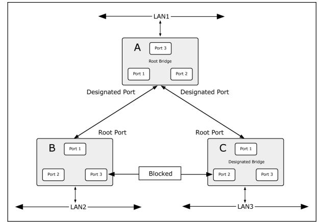
Figure 4-6-3 After Applying the STA Rules
