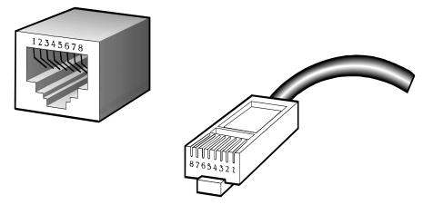
The standard RJ-45 receptacle/connector
