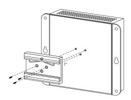
Step 2: Lightly insert the button of DIN-rail into the track
