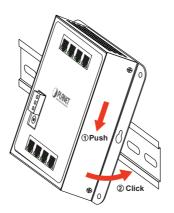
Step 3: Check whether the DIN-rail is tightly on the track
