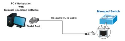
Figure 4-1 Managed Switch Console Connectivity
