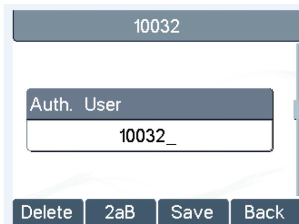
The screenshot shows a configuration screen for Authentication Name. At the top, a grey header bar contains the number "10032". Below this, a dark grey label "Auth. User" is positioned above a white text input field containing "10032\_". At the bottom of the screen, there is a dark grey bar with four buttons: "Delete", "2aB", "Save", and "Back".
