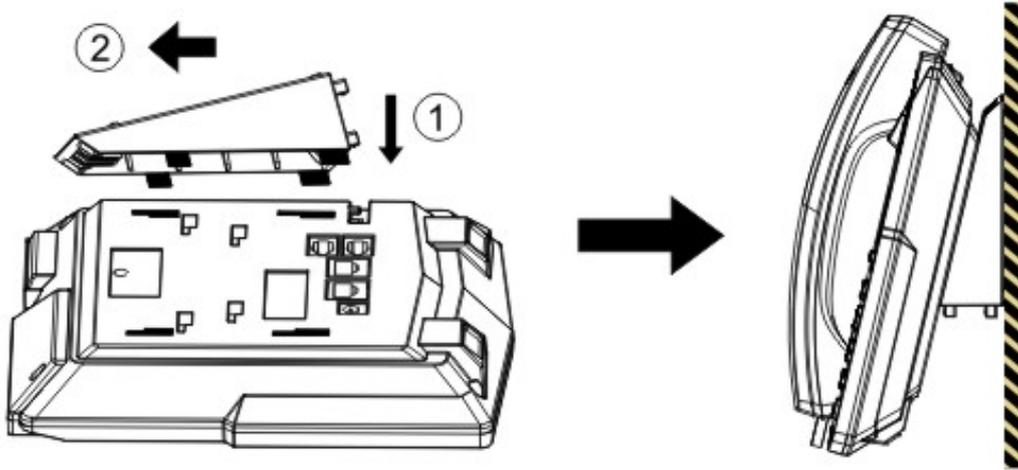
**Figure 4 - Wall-mount Installation**
