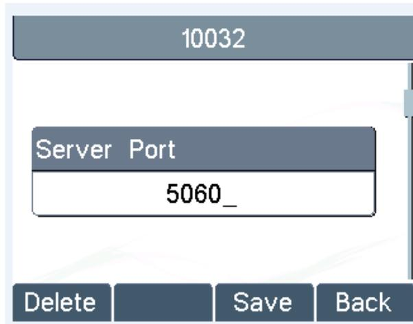
The screenshot shows a configuration screen for SIP Proxy Server Port. At the top, a grey header bar contains the number "10032". Below this, a dark grey label "Server Port" is positioned above a white text input field containing "5060\_". At the bottom of the screen, there is a dark grey bar with four buttons: "Delete", "Save", and "Back".
