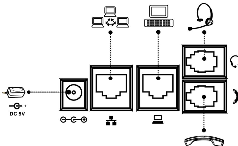
*Figure 2 - Connecting to the Device*
