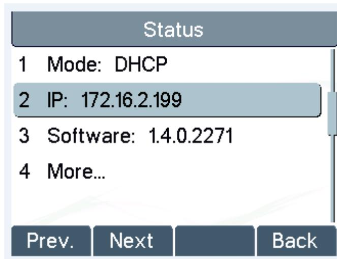
**Figure 7 - Check the Device's IP Address**
