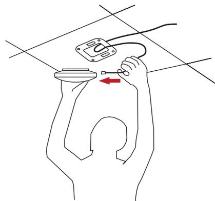
**Step 3:** Plug the other end of the Ethernet cable into the PoE switch.
