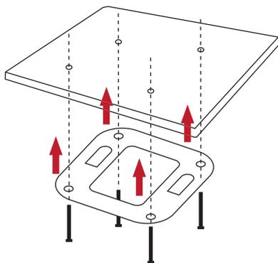
**Step 2:** Load the device into the mounting bracket, and be sure the device is mated with fixed screws. Then, lock the device in position and plug the Ethernet cable into the WNAP-C3220E.
