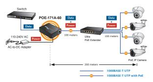
Figure 5: Connected Architecture over POE-171A series and POE-E304
