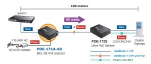
Figure 4: Connected Architecture over POE-171A series and POE-172S
