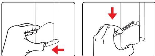
**Step 2:** Plug the RJ45 Ethernet cable into the PoE Port of the Outdoor Wireless CPE. Then, slide back the cover to finish the installation.
