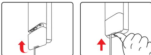
**Step 3:** Place the mounting strap through the slot on the back of the Outdoor Wireless CPE and then around the pole. Tighten the mounting strap to secure the Outdoor Wireless CPE.
