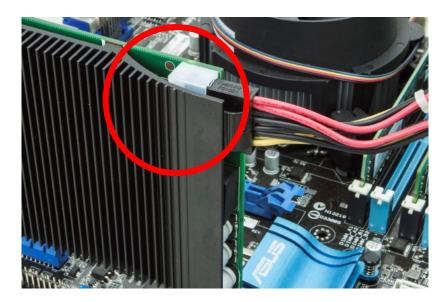
Step 5: If the ENW-9740P is installed, please plug in firmly the 4 Molex plug from power supply.
