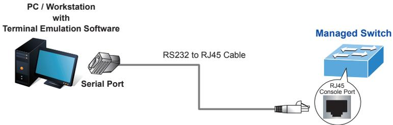
Figure 4-1 Managed Switch Console Connectivity
