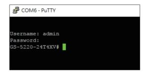
Figure 3-3: Managed Switch Console Login Screen
