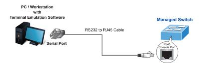
Figure 3-1: Managed Switch Console Connectivity
