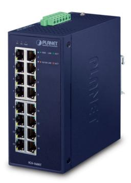
PLANET IGS-1600T Industrial high-density 16-port 10/100/1000T Gigabit Ethernet Switch is equipped with a rugged IP30 metal case for stable operation in heavy industrial demanding environments. Thus, the IGS-1600T provides a high level of immunity against electromagnetic interference and heavy electrical surges which are usually found on plant floors or in curbside traffic control cabinets.
