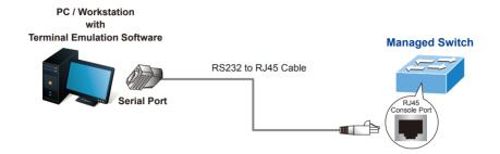
Figure 4-1: L3 Managed Switch Console Connectivity
