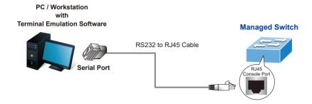
Figure 4-1: L3 Managed Switch Console Connectivity
