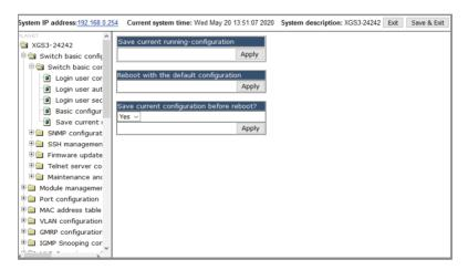
Press the "Apply" button to save current running-configuration to start up configuration.
