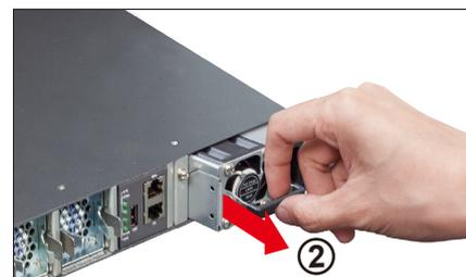
**Figure 4-1** Removing the Power Supply Unit
