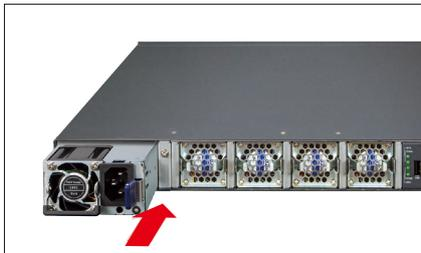
**Figure 3-3** Tightening the Thumbscrews
