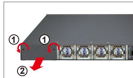
**Figure 3-1** Removing the Blank Plate
