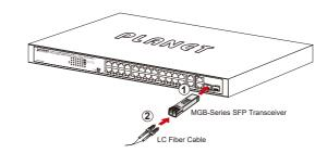
Figure 5-3: Plugging In the SFP Transceiver
