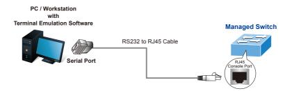
Figure 3-1: Managed Switch Console Connectivity
