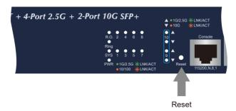
Figure 5-1: MGS-6320 Series Reset Button
