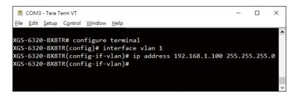
Figure 3-5: Configuring IP Address Screen
