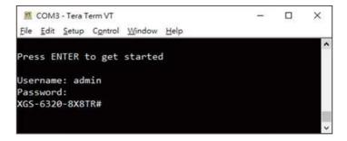
Figure 3-3: Managed Switch Console Login Screen
