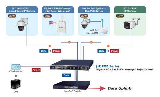
With data and Power over Ethernet from one unit, the (H)POE Managed PoE Injector Hub series can reduce power cable deployment and eliminate the need for dedicated electrical outlets on the wall, ceiling or any unreachable place.
