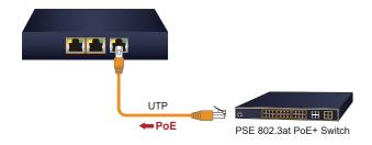
Step 2: The PSE delivers both Ethernet Data and PoE power over UTP cable to the Gigabit PoE Extender and the "PoE-in-use" and "LNK/ACT LED" will be lit steadily.
