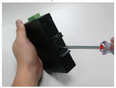
Step 2: Lightly slide the DIN-rail bracket into the track.
