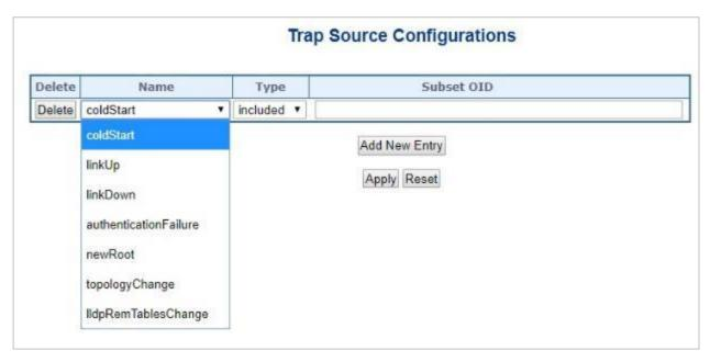
Figure 4-2-2-6: SNMP Trap Source Configuration Page Screenshot
