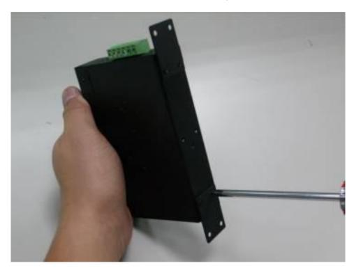
Step 3: Use the screwdriver to screw the wall mount plate on the Industrial Managed PoE+ Switch.
