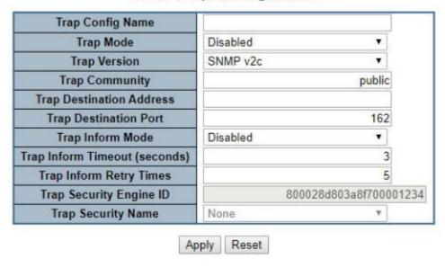
Figure 4-2-2-4: SNMP Trap Configuration Page Screenshot
