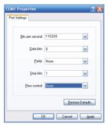
Figure 4-2: COM Port Configuration
