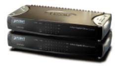
The GSD-504 / GSD-804 are 5/8-Port 10/100/1000Mbps Gigabit Ethernet switches in compact housing for easily desktop deployment.
