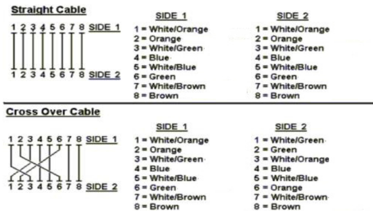
Figure A-1 Straight-Through and Crossover Cable
