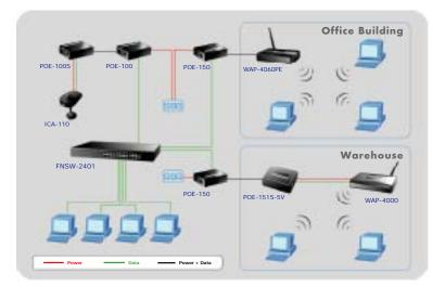
To control the power system of your networking devices, POE-151S can be installed and co-work with the third party 802.3af POE injector hub such as building VoIP telephony network in the office. Besides, the POE-150 can be directly deployed to connect the third part 802.3af devices installed 100 meters away.
