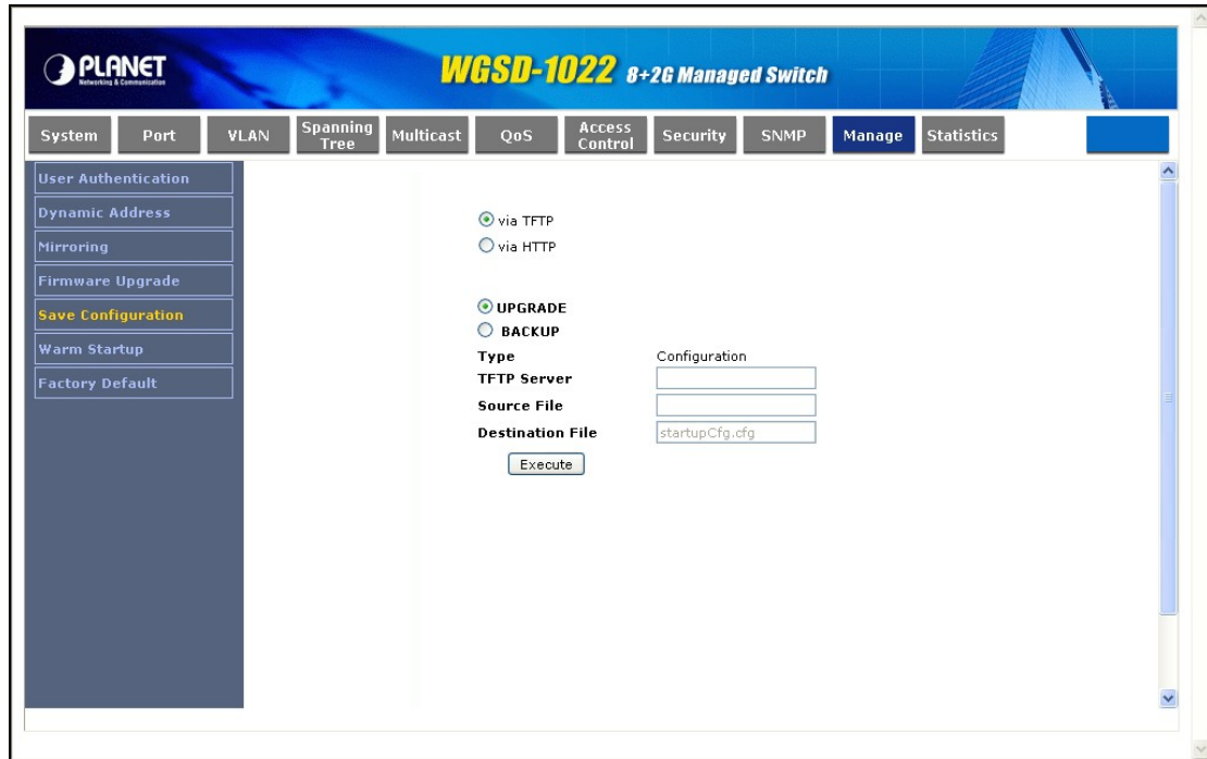
Figure 4-58 Save Configuration via TFTP
