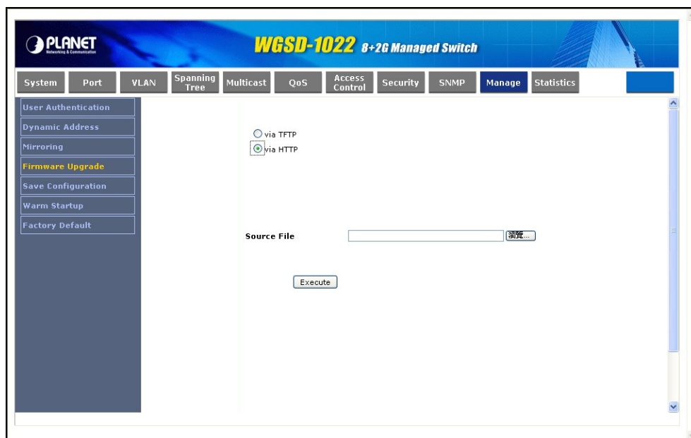
Figure 4-57 Firmware Upgrade via HTTP
